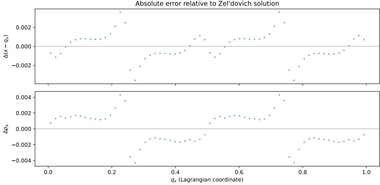
Figure 20.5.: Absolute error in displacement and momentum relative to the exact Zel'dovich solution. The errors combine both time-stepping error and spatial PM error (CIC window, discrete grid). See the convergence tests below to disentangle these contributions.
